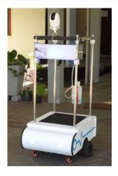
robot unit is designed by **NERD** Centre to assist doctors & other medical staff who are engaged in of covid-19 treating patients. Use of this unit provides multiple advantages such doctors or medical staff can inspect the ward through tab screen; the trolley movement can
